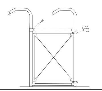
Attach the GATE LATCH (L) to the GATE DOOR at a comfortable and desired height. Cover the entire GATE DOOR with your fencing mesh (NOT INCLUDED) and fasten the mesh to the GATE DOOR using SELF-LOCKING TIES (O). Trim excess as needed.
